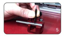
Remove the split pin by inserting the assembly tool and drive it slowly out of the tool body with a small hammer.
