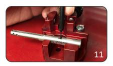
Place the tool body on the front bed of the mounting fixture and insert the split pin with the assembly tool and a small hammer.
