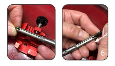
Push the spring back – at the front edge of the spring – over the pre-loaded split pin by using the pin of the mounting fixture first and then the assembly tool pin.
