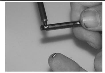
1. Press the rollpin from the side without groove carefully out of the tool body by using the assembly pin – if necessary by using the hammer too.
