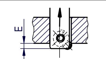
1. Rapid traverse of the cutting unit of the tool **above** the top material surface of hole or burr. Referencing the front edge of the cutting blade.
