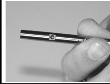
1. Insert the spring from below into the tool body. Note that the spring index must be visible.
