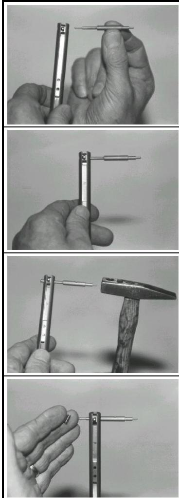
1. Position the assembly pin in a way that the longer side points to the tool.
