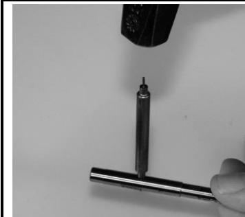
1. Push the assembly pin with the shorter side into the bore opposite as shown on the picture.
