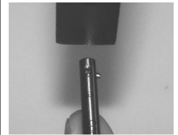
1. Insert the COFA blade into the tool with notch (blade groove) towards the spring => note the marks illustrated on the tool body
