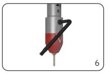
To complete the blade change, tighten the clamping screw using the Torx wrench.
