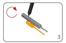
Insert a small pointed instrument through the hole on the underside of the blade housing. This lifts the blade out of its housing enabling easy removal.
