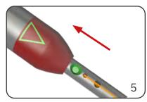
Slide the blade housing back into the tool body. The arrow on the coolant sleeve is aligned with the bore of the clamping screw.
