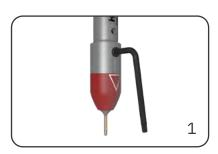
Loosen the clamping screw with the supplied Torx wrench.
