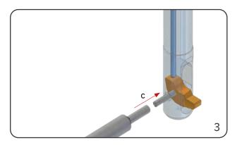
**Assembling** – Insert the blade. Then insert the split pin with the flat end of the assembly pin first and position the blade (c).
