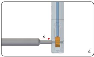
Push the split pin with the non-stepped end of the assembly pin until it is flush with the blade housing (d). Blade is fixed in place. Carry out function check.
