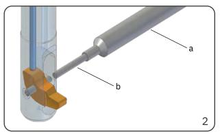
Use the stepped end (b) of the assembly pin and position the assembly pin with the slot free end onto the split pin. Press the assembly pin in until the split pin falls out and the blade is free to be removed.
