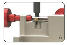
Guide the assembly pin with its long end through the bore and center the blade.
