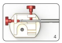
Push out the blade by means of the long end of the assembly pin.
