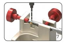
Insert the split pin manually with the split end upwards. Then push it with the assembly pin.
