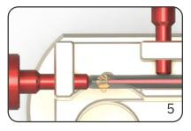
Insert the new blade into the tool with the blade groove orientated towards the spring. Please observe the marks on the tool body.
