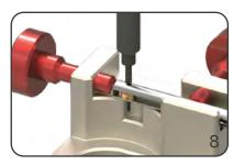
The assembly pin must be level with both sides of the tool body.
