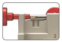
Adjust the tool lengthwise so that the blade bore is above the recess for the split pin. Clamp the tool as shown.
