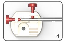
Push out the blade by means of the long end of the assembly pin.
