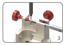
Push the split pin carefully out of the bore. Make sure you apply the assembly pin to the split end of the pin. If necessary, use a small hammer.
