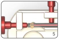
Insert the new blade into the tool with the blade groove orientated towards the spring. Please observe the marks on the tool body.
