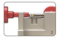
Adjust the tool lengthwise so that the blade bore is above the recess for the split pin. Clamp the tool as shown.
