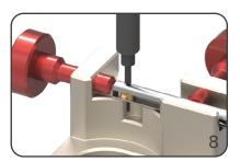
The assembly pin must be level with both sides of the tool body.
