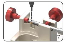
Insert the split pin manually with the split end upwards. Then push it with the assembly pin.
