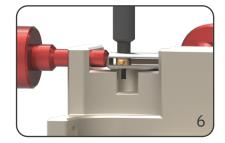
Guide the assembly pin with its long end through the bore and center the blade.
