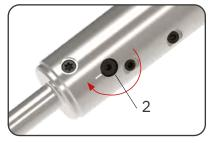
Turn the eccentric cam (2)back to the left until a slight resistance is noticed. Finally, both markings are next to each other.
