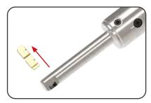
Remove blades from blade housing (by pushing).
