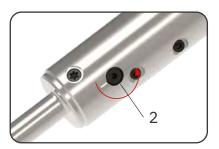
Turn the eccentric cam 180° until the notch is facing opposite of the index.
