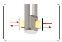
**Check:** Press both blades with thumb and index finger together. Both blades must move synchronously.
