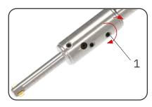
Continue to turn tension screw (1) clockwise until the desired blade force is attained. The previously set chamfer size remains the same before and after changing the blades. For reference values for the blade force please refer to page 109.
