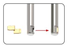
Insert the replacement blades as a pair, cleaned and so that they are approximately flush with the outside diameter of the blade housing.
