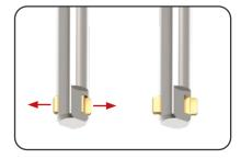
Move the inserted blades outwards (arrow) until they engage automatically.
