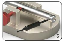
Use larger diameter of assembly pin to push the blade out of the blade holder.
