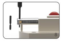
Insert new split pin short section first into the hole until the back end of the pin is flush with tool holder.
