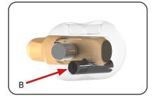
Place tool into the assembly device so that support pin from the assembly device enters into the spring recess behind the fixing strip and that the tool holder lies with its contour flush on the front rest.
