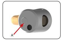
Assembly device for tool types COFA C6 - C12 Note: Execute blade change on mounted tool only.
