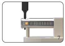
In order to define the right position of the blade and to pre-center for the new split pin, push the assembly pin in the split pin hole.
