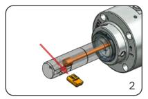
Push out the blade. Keep the buttons pressed until the blade is completely removed.
