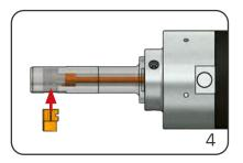
Insert blade in blade window to the extent that the cutting part of the blade remains fully visible. To do this keep on pushing the buttons of the control unit.
