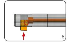
Position the blade in the blade window so that the blade control pin audibly engages into the blade.
