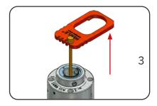
Pull forward the blade control too by applying some force but without unscrewing anything.
