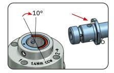
Mount the blade housing onto the control unit. Please make sure that the blade control bolt is mounted with a twist of approx. 10° into the clearance groove of the blade housing.
