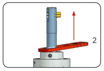
Pull the blade housing forward away from the control unit. The blade house wrench simplifies the disassembly and should be used always.
