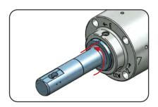
Then, align the mark of the blade housing with the mark of the control unit.
