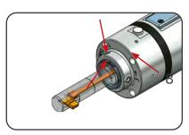
Screw the 3 clamp screws tightly. For this, please observe the torque value and screw order indicated on the control unit housing.
