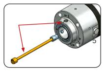
**Assembly:** Push blade control (snap mechanism + seal) well positioned with some force into the control unit. **Attention:** Please make sure that the mark on the blade control and the mark on the control unit are aligned.
