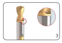
There should be a seamless transition between drill bit and tool body after the tightening of the drill bit (no light gap between tool body and drill bit).
