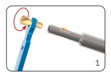
Unfasten the drill bit with a flat wrench in counter-clockwise direction from the tool body.
