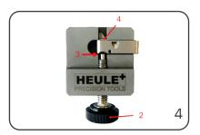
Tighten the adjusting screw (2) of the assembly fixture until the edge of the module (3), the breaking edge (4) of the assembly aid is visible.
