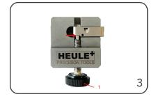
Tighten the adjusting screw (1) of the assembly fixture until the blade window clearance of the module.
