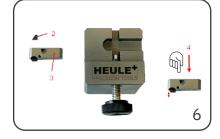
Untighten the adjusting screw, dispose of the assembly aid (2) properly and take out the module (3)
