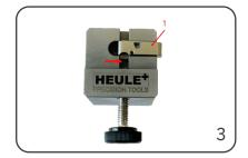
Insert the module with the blade (1) into the assembly fixture, the chamfer blade is pointing towards the adjusting screw.
