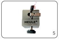
Break off the assembly aid with the mounting pin (1) (apply gentle pressure with the tip on the assembly aid).
