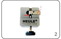
Insert the module with the blade (4) into the assembly fixture, the chamfer blade is pointing towards the adjusting screw.
